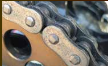
rust on pin/plate surface
